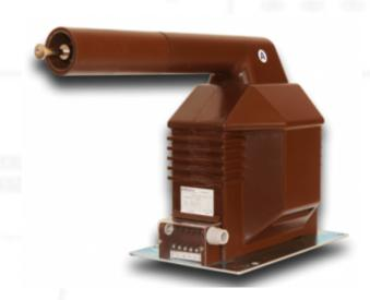
Voltage instrument transformers VTS 36P are single-phase transformers isolated with one pole. They are designed for the use in the high voltage systems from 15 kV to 38.5 kV. They are designed for measuring and protection of high voltage distributing equipment for indoor design. The instruments are equipped with high voltage fuse protecting the surrounding distributing system.
